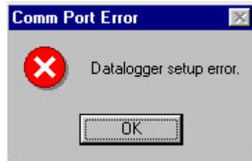
check that all the connections are correct, including that the correct serial port has been selected and that no other software has control of this serial port. Make sure that the batteries are charged. Disconnect and reconnect the battery pack while the serial cable remains connected and try the setup procedure again.
